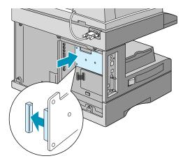
**11** Insert the teeth at the bottom of the control board cover into the corresponding slots on your machine.
